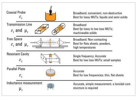
Figure 1. Materials measurement techniques
